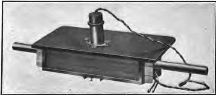
FIG. 104.—Scale Box with Lamp, for Torsionmeter.
